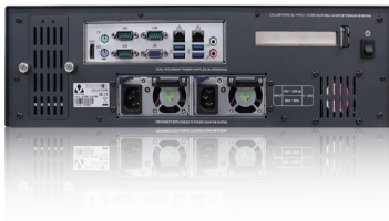
Rear view (above) showing dual Gig-E ports, alarm/relay connections and the dual hot-swap PSU option. Note that the two cooling fans are software controlled and are normally switched off.
