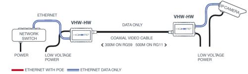
HIGHWIRE devices are used to convert conventional Ethernet to a signal that can be carried by 75ohm coaxial cables such as RG59, RG6 and RG11.
