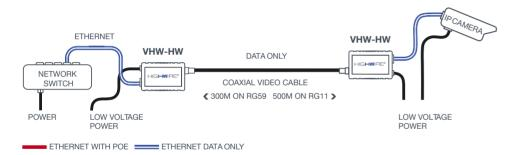
HIGHWIRE devices are used to convert conventional Ethernet to a signal that can be carried by 750hm coaxial cables such as RG59, RG6 and RG11.
