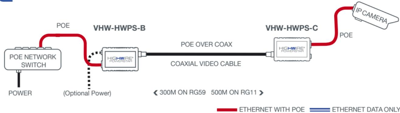
HIGHWIRE Powerstar Base and Camera devices are used together to adapt conventional Ethernet to a signal, with POE, that can be carried by coaxial video cables such as RG59.
