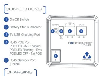
POINTSOURCE Plus should be charged before first use and after long periods of storage. If stored, it should be fully charged before storage, and recharged every 6 months to maintain battery performance.
